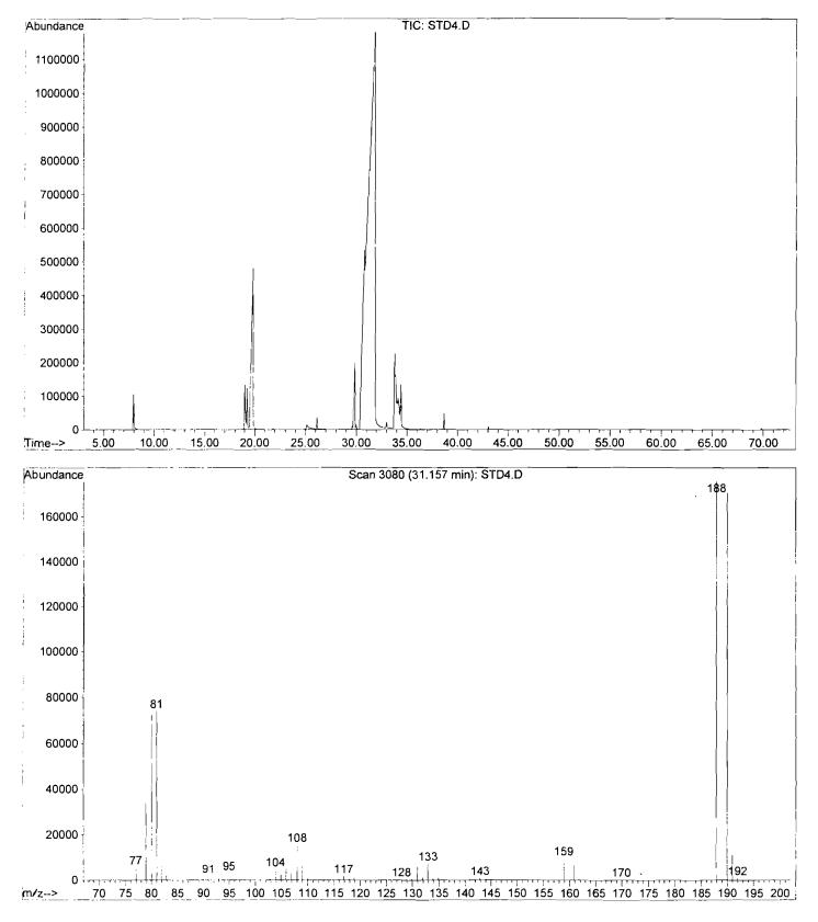
File : C:\HPCHEM\1\DATA\STD3.D Spectrum  $\lambda$ Operator : Kris Mitchell Acquired : 6 Oct 97 11:08 am using AcqMethod INVERT Instrument : GC/MS Ins Sample Name: 2,4,6 tribromo phenol Misc Info : .1 g of each in 40 mLof methanol Vial Number: 1
