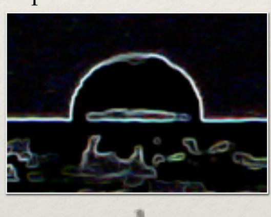
Then we randomly sample nearly- or pure-white pixels which could potentially be points on the circle (i.e., the drop).
