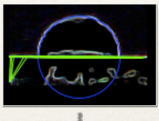
The geometry of the detected circle and surface is analyzed to determine the angle of contact between the two.
