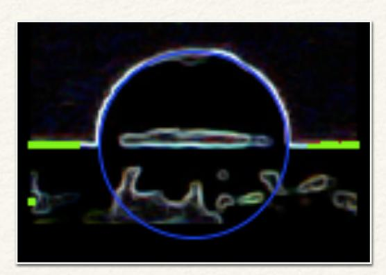
To locate the surface on which the drop rests, we collect the light pixels outside the circle.
