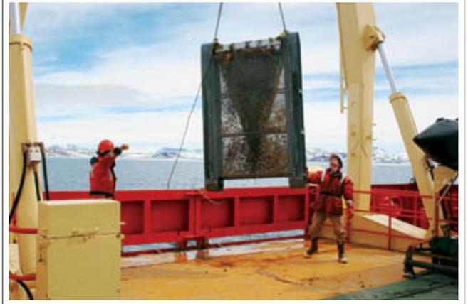
Collections of bottom-dwelling invertebrates were made with dredges such as the epibenthic sled (above) that is lowered onto the ship’s deck. (Photo by E. Balser)
