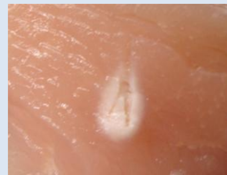
Cross-section of RF lesion caused using a protruding electrode (18 g) at 80 °C for 90 s.
