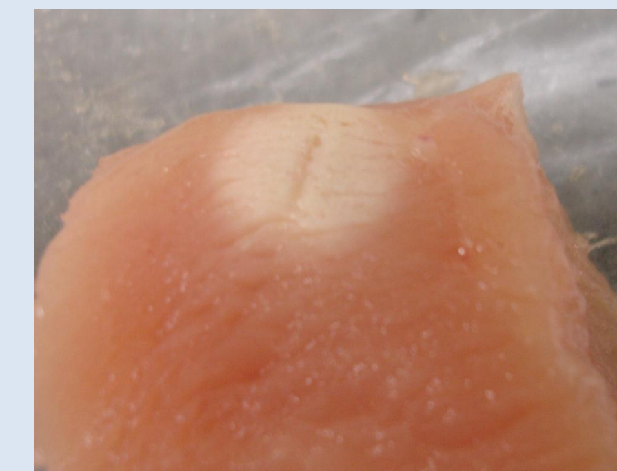
Cross-section of RF lesion caused using a cooled tip at 60 °C for 150 s.
